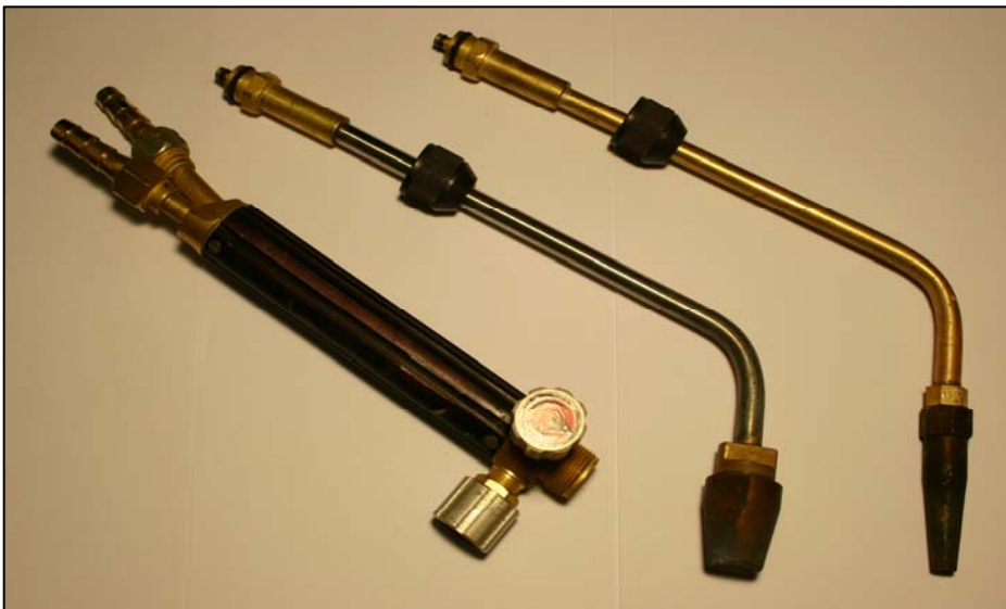
Fig.8. Parts of torches brazed with the filler metal P14
