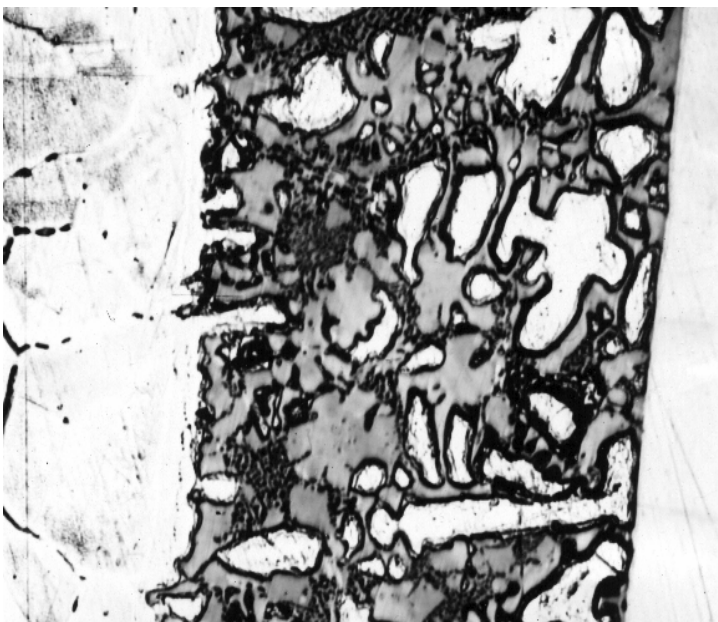
Fig. 3 Microstructure of a brass-to-steel joint brazed by the filler metal P81. x120
