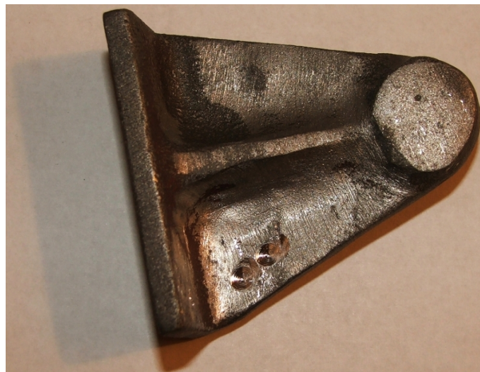
Fig. 2 A cast article with the defects prepared for soldering
